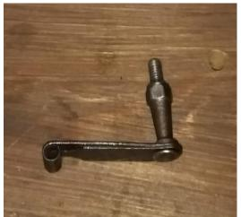
This is the clip fitted to the bike. The spring arm is too short and the stub on the spring arm fails to reach the dimple in the centre of the cover.
