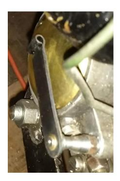
The finished clip in place. It fits nicely with a nice, positive feel when the stub engages with the dimple in the points cover.
